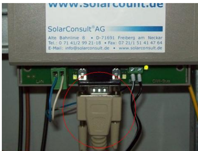
Abb. 4 Anschlüsse am SolarCount Net
